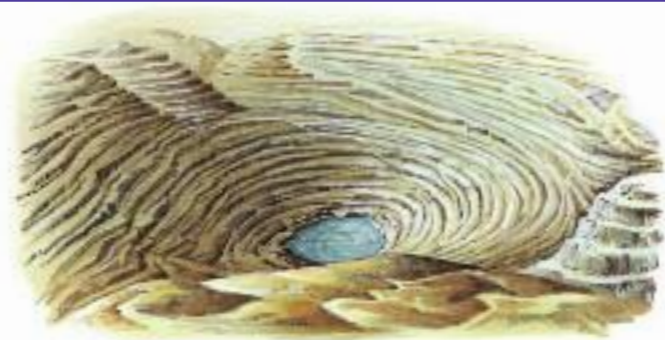
This is an opencast copper mine. Huge excavators cut away the surface rock and dig up the ore.
